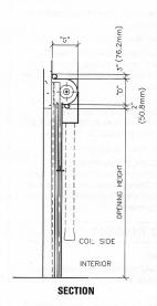
3" (76.2 mm) is dimension of top hood bead. Where headroom is limited, 3" (76.2 mm) requirement can be eliminated by turning bead down.
