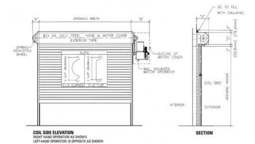
3" (76.2 mm) is dimension of top bead. Where headroom is limited, 3" (76.2 mm) requirement can be eliminated by turning bead down.
