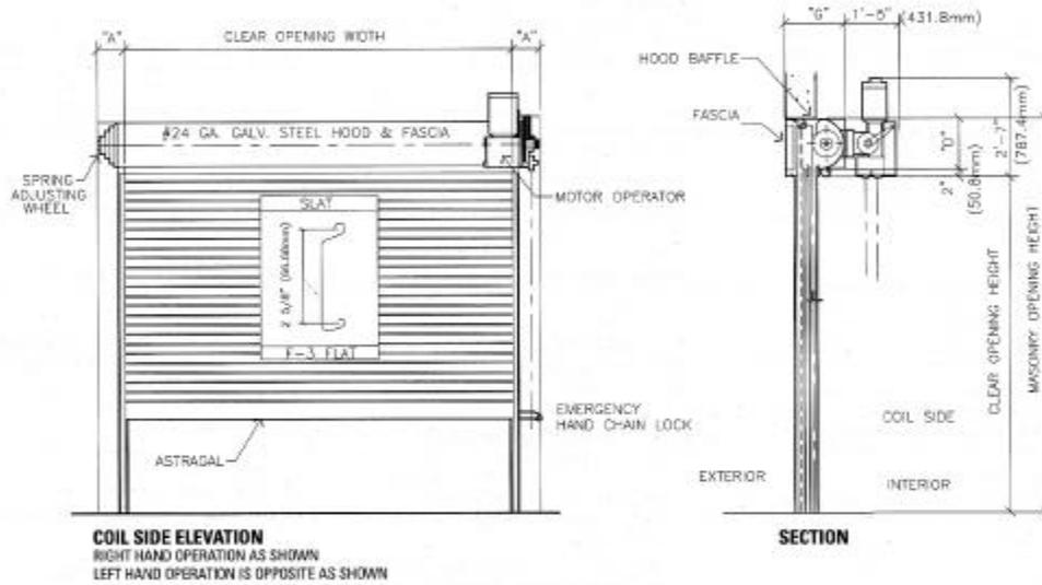
Windlocks are standard on doors over 18'-4<sup>1</sup>/<sub>8</sub>" (5610 mm) wide and optional for doors under 18'-4<sup>1</sup>/<sub>8</sub>" (5610 mm) wide.
