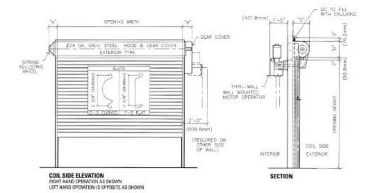
3" (76.2 mm) is dimension of top hood bead. Where headroom is limited, 3" (76.2 mm) requirement can be eliminated by turning bead down.
