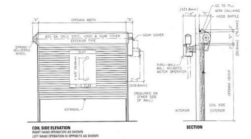
3" (76.2 mm) is dimension of top hood bead. Where headroom is limited, 3" (76.2 mm) requirement can be eliminated by turning bead down.
